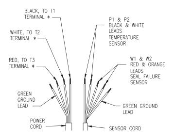
\* TERMINALS T1, T2 AND T3 IDENTIFY MAGNETIC STARTER TERMINAL CONNECTIONS.
