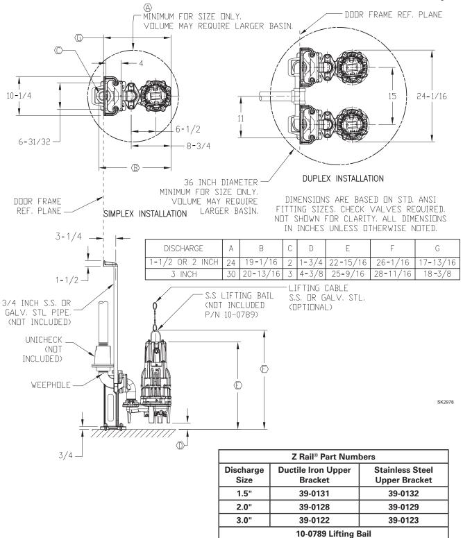
\*Intermediate rail bracket required every 12' of basin depth. Refer to ZM1347
